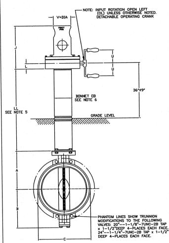
NOTE: DIMENSION "C" ALLOWS CLEARANCE FOR 150 LB OR 125 LB A.S.A. BOLT LAYOUT.
