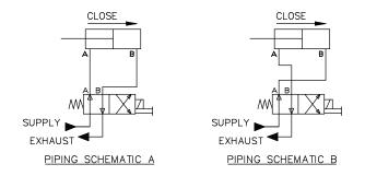
PIPING TO 4-WAY VALVE PORTS "A" & "B' CAN BE REVERSED AS SHOWN IN PIPING SCHEMATIC "B" (IF REQUIRED)
