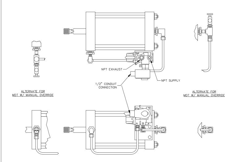
ELECTRICAL CHARACTERISTICS (UNLESS OTHERWISE NOTED) 120 V AC 20 WATTS
