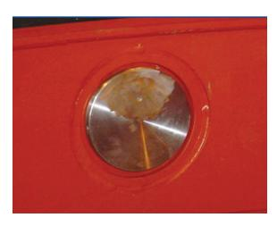
The Pk Posi-Loc positively mechanically locks a butterfly valve disc in the closed position.
